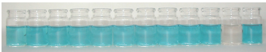
Figure 8.4 Receptor 8.53 in acetonitrile ( [\text{8.53}] = 3.0 \times 10^{-5} \text{ M} ) in the presence of 5 mol equiv. of various anions; from left to right, \text{F}^- , \text{Cl}^- , \text{Br}^- , \text{I}^- , \text{NO}_3^- , \text{H}_2\text{PO}_4^- , \text{HSO}_4^- , \text{Ac}^- , \text{Bz}^- , \text{SCN}^- , \text{CN}^- , and no anion. (Reproduced with permission from ref. 60 Copyright 2002 Royal Society of Chemistry)
